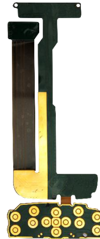
10L Rigid-flex PCB Application: Industry Control Buried via hole
